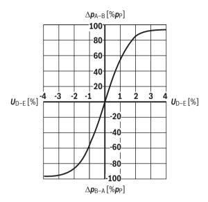
Pressure/signal characteristic curve (symbol V)
